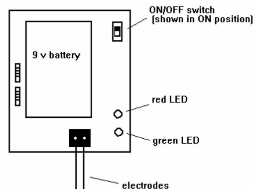
All you need to do is pick up the device and place the two metal electrodes sticking out from one end into the solutions you prepared earlier in the wells. You should rinse the wires off between solutions with a squirt of distilled water. Record your conductivities in relative terms (no light = no conductivity, red = fair, red and green = good). You should also test tap water and distilled water just to have some kind of comparison.
