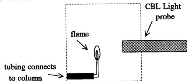
The CBL light probe is sensitive to both visible and infra-red radiation. The flame is initially adjusted to be small and nearly all blue so that mostly infra-red radiation is emitted. When one of the alkane isomers emerges at the end of the column it too burns, increasing both the luminosity and heat of the flame. The light probe converts this into a voltage which it sends to the CBL.
