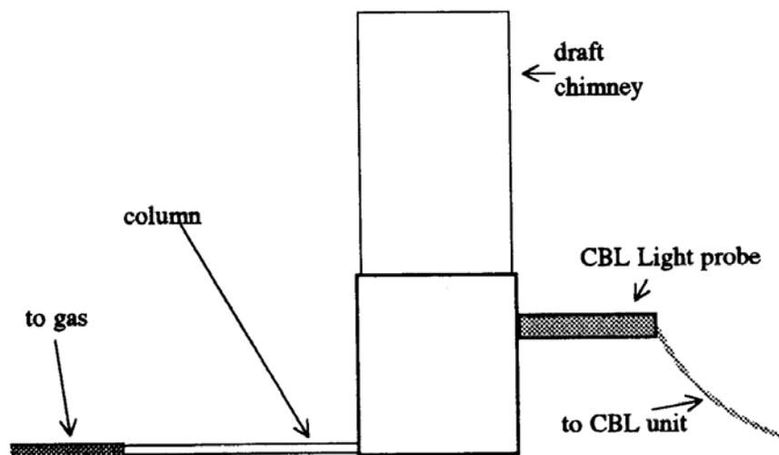
The column is made from glass tubing that has been filled with Tide<sup>®</sup> laundry detergent. The detergent contains many different kinds of compounds but the actual detergent molecules are structured to have one end that is polar and one that is non-polar:
