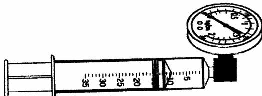
The syringe is connected to a pressure gauge and about 30 mL of air has been trapped in the syringe at atmospheric pressure ( $\approx 1$  atmosphere). The gauge reads *additional* pressure and the inside scale is in atmospheres. By changing the volume of the trapped air sample you can determine how the pressure is affected.
