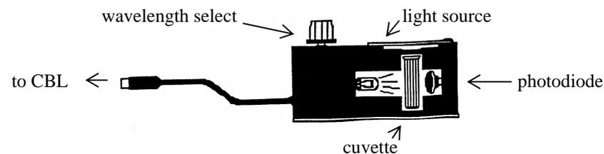
The wavelength select knob has a setting for 0% transmittance which is used during the calibration routine run by the program in your calculator. The light selection is also made with this knob which is turned to the wavelength (color) that will be most strongly absorbed by the solution.
