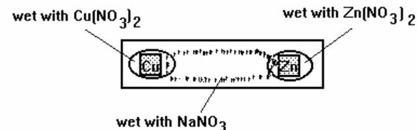
[the  $\text{NaNO}_3$  in the middle of the strip acts like the "salt bridge" or U-tube in the traditional set-up, allowing ions to migrate slowly across the paper, maintaining the electrical connection]
