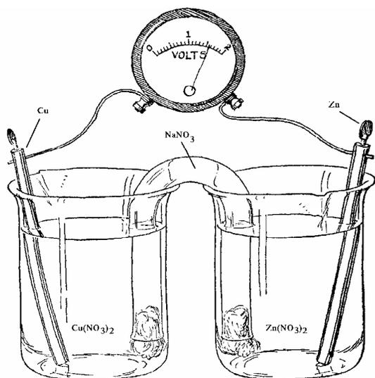
This *looks* very nice but in practice gives rather poor results and uses a lot of solutions. You can achieve far better results and use up less material by placing two pieces of metal at opposite ends of a strip of filter paper that has been wet with the appropriate solutions:
