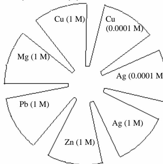
By placing metal pieces on drops of their ionic solutions and "bridging" the gap in the center with  $\text{NaNO}_3$  you can easily set up a number of different reactions to investigate.
